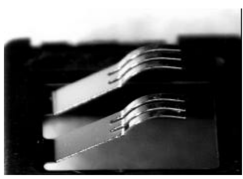
Figure 7: View of recent design, dual trace thick film sensor a) top view b) contact assembly
