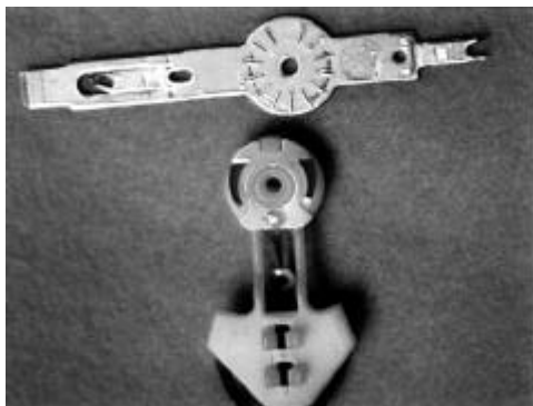
Figure 5: View of early generation single trace thick film sensor a) top view b) contact assemblies
