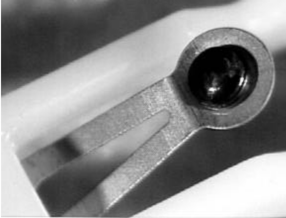
Figure 13. Typical geometry for a mechanically staked rivet contact. When this style contact is used in a sliding application, it usually represents the only point of contact to the conductive inks.
